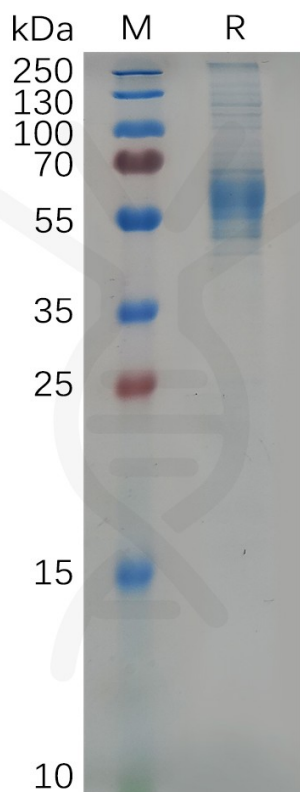
Figure 1. Mouse CD123 Protein, His Tag on SDS-PAGE under reducing condition.
