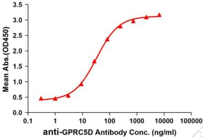
Figure1. Elisa plates were added with Flag Tag GPRC5D-Nanodisc (0.5 $\mu$ g/per well) on an anti-Flag monoclonal antibody pre-coated (0.5 $\mu$ g/per well) plate. Serial diluted anti-GPRC5D monoclonal antibody (DME100090) solutions were added, washed, and incubated with secondary antibody before Elisa reading. From above data, the EC50 for anti-GPRC5D monoclonal antibody binding with GPRC5D-Nanodisc is 32.86ng/ml.
