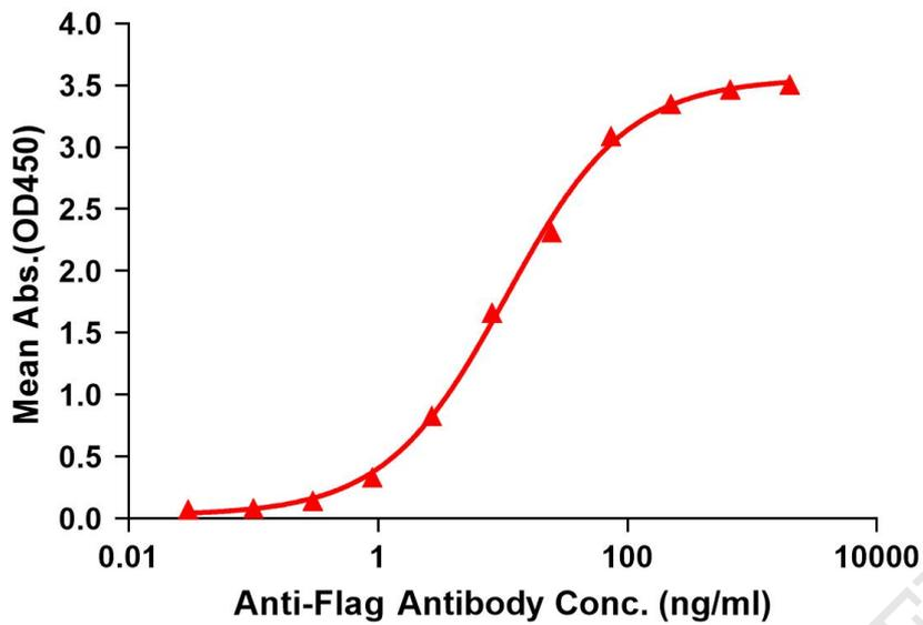
Figure 1. Elisa plates were pre-coated with C-Flag&Strep Tag GALR1-Strep-Nanodisc (0.2 $\mu$ g/per well). Serial diluted anti-Flag monoclonal antibody solutions were added, washed, and incubated with secondary antibody before Elisa reading. From above data, the EC50 for anti-Flag monoclonal antibody binding with GALR1-Strep-nanodisc is 10.66ng/ml.
