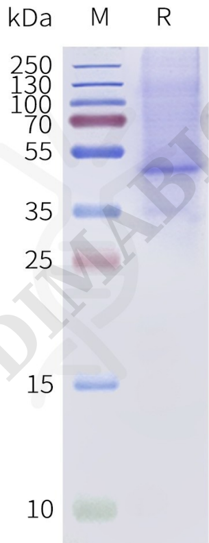
Figure 2. Human BRIL-MC2R-Strep-Nanodisc, C-Flag&Strep Tag on SDS-PAGE
