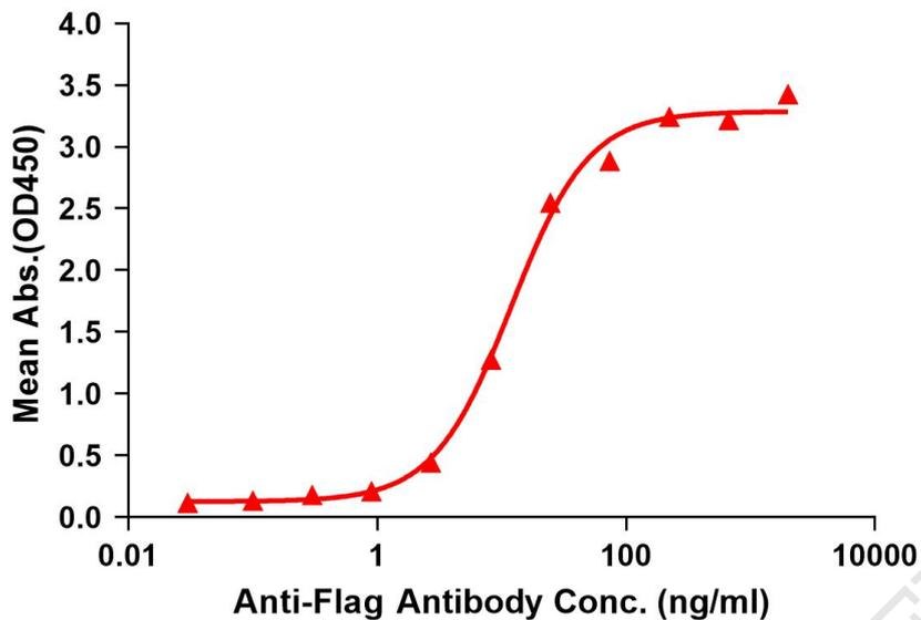
Figure 1. Elisa plates were pre-coated with C-Flag&Strep Tag ACKR1-Strep-Nanodisc (0.2 $\mu$ g/per well). Serial diluted anti-Flag monoclonal antibody solutions were added, washed, and incubated with secondary antibody before Elisa reading. From above data, the EC50 for anti-Flag monoclonal antibody binding with ACKR1-Strep-nanodisc is 11.96ng/ml.
